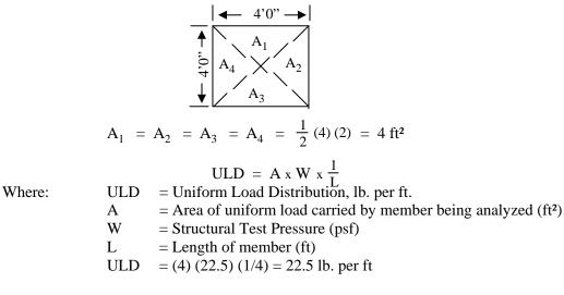
A. Based on the above tested unit, will a 3' 0" x 5'0" fixed unit meet R15?
